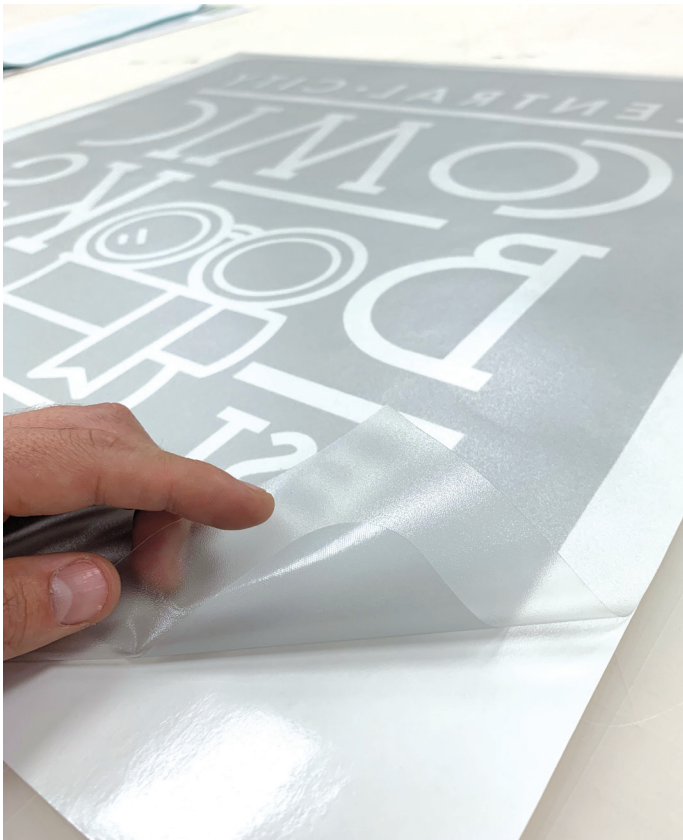
Step six: the vinyl needs to be transferred from the backing paper it is currently on to the surface of the acrylic.
