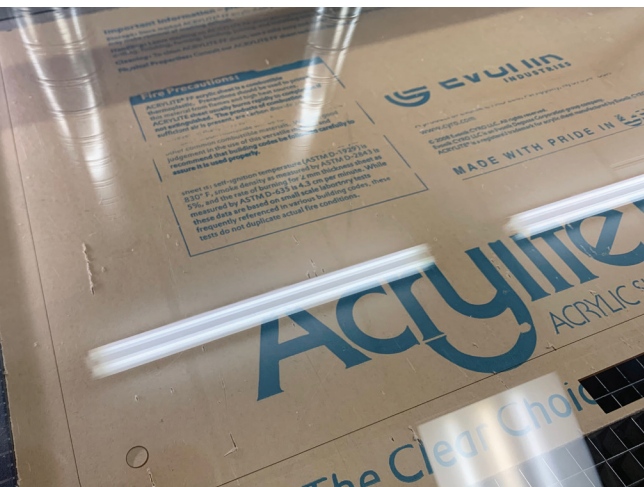
Step two. When cutting acrylic and hardboard, it's best to use a slow speed and high power setting with multiple passes.
