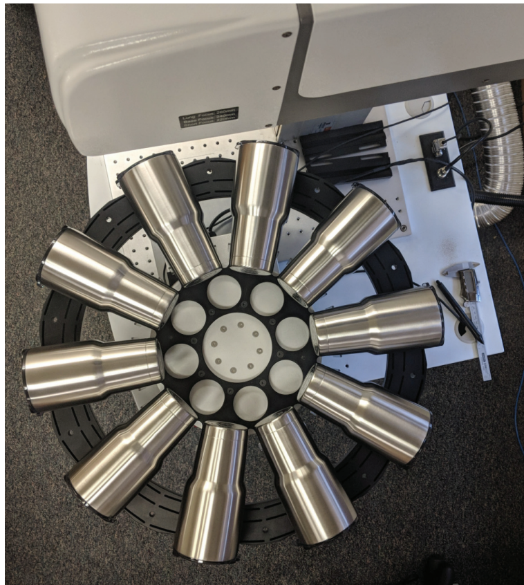
The disc rotary system and drinkware nest allows users to load up to 10 30-ounce cups and let the rotary cycle them through while working on other tasks.
