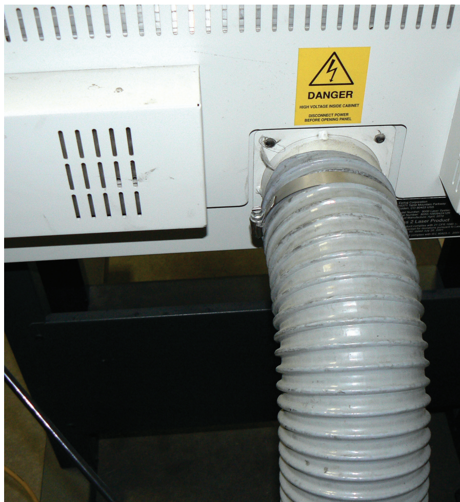
The laser outside exhaust vent and hose leading to my exhaust filtering system – it's crucial to keep your vent clean. ALL IMAGES COURTESY BOB HAGEL
